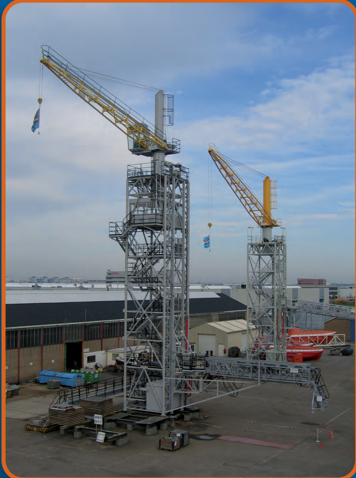
All Verhoef Access Systems are shop-erected and fully tested before delivery, guaranteeing a quick commissioning of the equipment at site.
